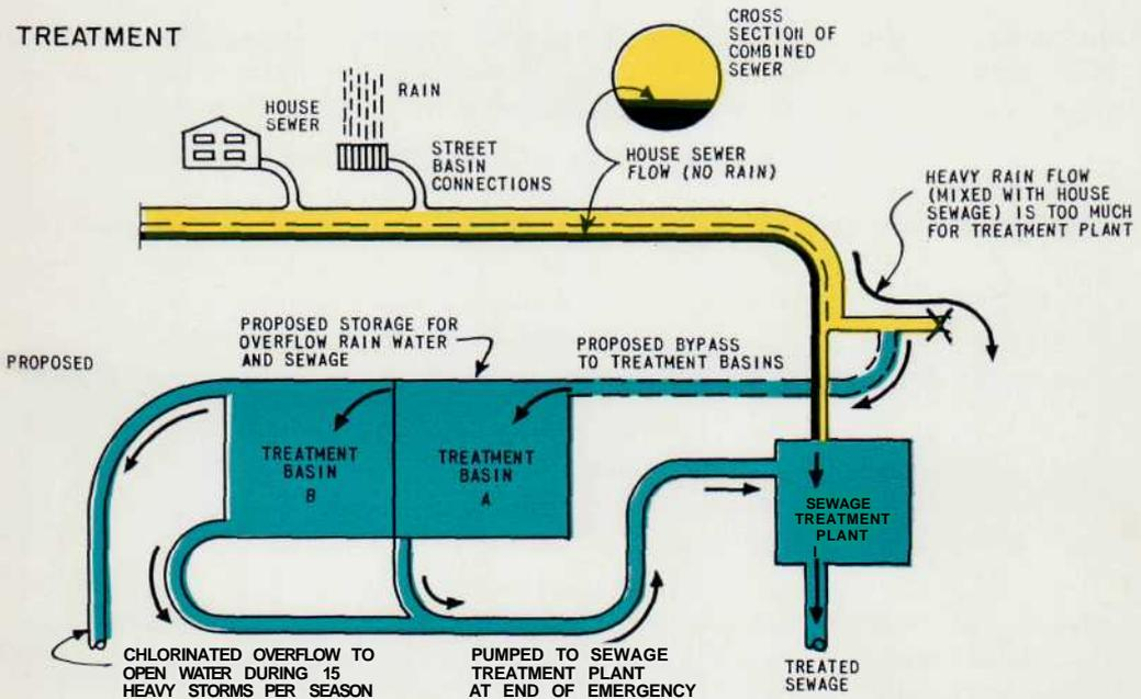
Diagram showing (at top) the difference between a combined sewer; and separate sewers for house sewage and rainfall; and the proposed remedy in certain areas. The marginal problem is the overloading of the system when heavy rain falls. At bottom is diagram of proposed treatment basins where overflow is stored and settled for treatment after emergency. If load is too heavy overflow is chlorinated.
